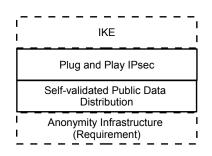
**Fig. 2.** The layering of our protocols (boxed with solid lines) and related protocols (boxed with dashed lines).
