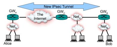
Fig. 4. PnP-IPsec Deployment Topology. Alice and Bob are communicating hosts; PnP-IPsec is deployed on  $\mathsf{GW}_A$  and  $\mathsf{GW}_B$  and establishes an IPsec tunnel between them.
