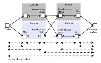
Figure 1: *Herd*'s architecture comprises clients, mixes located in trust zones, and optionally, SPs (not shown). *Herd* employs both hop-by-hop and layered encryption to hide content, routing information, and circuit IDs. Mixes can also act as rendezvous enabling clients to receive incoming VoIP calls with zone anonymity. Optionally, a caller and callee can use an additional zone (e.g., *A* and *B*) to avoid depending on the same jurisdiction.
