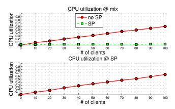
Figure 6: CPU utilization of a mix (top) and SP (bottom), as a function of the number of clients supported.
