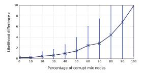
**Figure 8:** Likelihood difference  $\varepsilon$  depending on the percentage of (passively) corrupted mix nodes. We use  $\lambda = 2$ ,  $\mu = 1$  and a topology of 3 layers with 3 nodes per layer.
