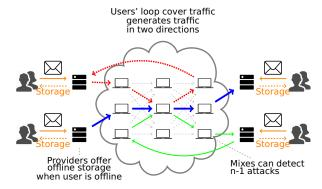
Figure 1: The Loopix Architecture. Clients pass the messages to the providers, which are responsible for injecting traffic into the network. The received messages are stored in individual inboxes and retrieved by clients when they are online.
