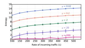
Figure 5: Entropy versus the changing rate of the incoming traffic for different delays with mean  $\frac{1}{\mu}$ . In order to measure the entropy we run a simulation of traffic arriving at a single Loopix mix node.
