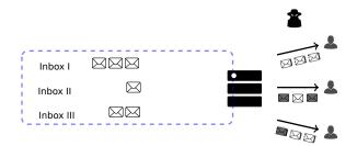
Figure 4: Provider stores messages destined for assigned clients in a particular inbox. When users pull messages from the mix node, the provider generates cover messages to guarantee that the adversary cannot learn how many messages are in the users inbox. The messages from the inbox and dummies are indistinguishable.
