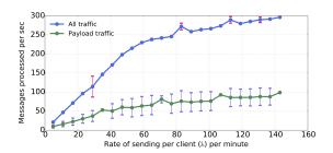
Figure 9: Overall bandwidth and good throughput per second for a single mix node.
