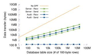
Figure 5: The total client and server data transfer scales sub-linearly with the size of the database.
