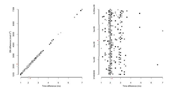
Figure 3.7: Time dependence of consecutive ISNs. Linux is shown on the left and random ISNs, with the same inter-packet timing, is on the right. The packets were sent approximately every 2 milliseconds, hence the clustering on the x axis around this point. The ISN difference is clearly correlated with inter-packet sending time for Linux, but uniformly distributed with random ISNs. Again point colour indicates packet ordinal
