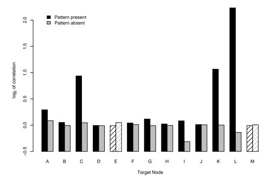
Figure 4.5: Summary of correlation. For each node, the left bar shows the correlation when the victim stream was travelling though the node (false negative test) and the right bar shows the correlation when it was not (false positive test). The two incorrect results (E and M), where the correlation was higher when the traffic was not being sent through the nodes, are highlighted with diagonal shading lines
