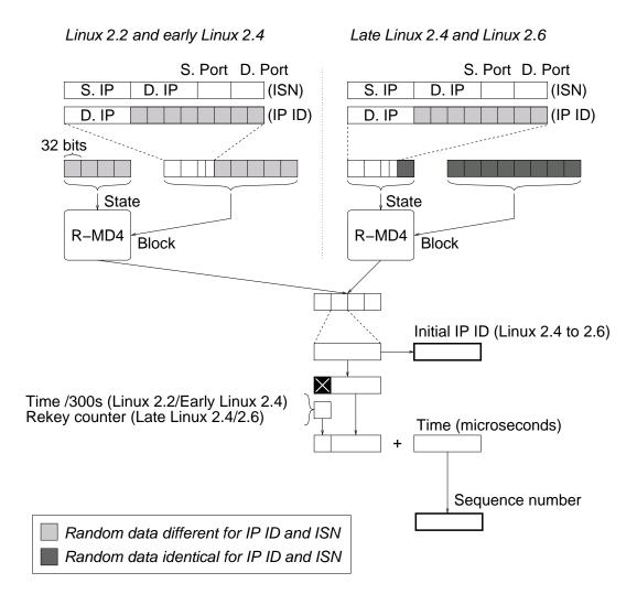
Figure 3.4: Linux 2.2–2.6 ISN generator and Linux 2.4–2.6 IP ID generator
