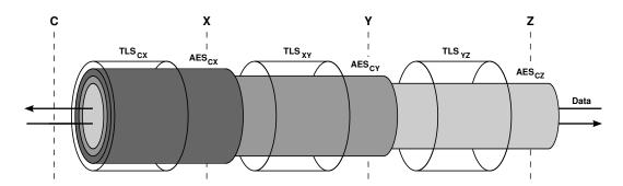
Figure 4.1: Encryption performed and key usage for a Tor circuit, going from the Onion Proxy C, through three Onion Routers: X, Y and Z.  $TLS_{ab}$  indicates the TLS tunnel secured by keys shared between a and b.  $AES_{ab}$  indicates the CTR mode encryption performed using a key shared between a and b
