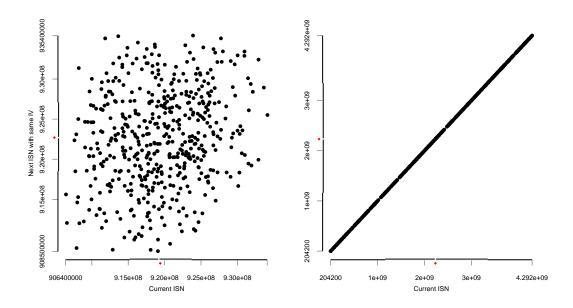
Figure 3.8: With Linux, shown on the left, there is no significant correlation between pairs of packets with the same Nushu ISN, other than that expected from the similar most significant byte. In contrast, for such packets, the Nushu generated ISN, shown on the right, is identical, assuming a constant payload
