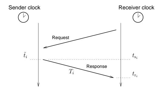
Figure 5.2: Time and timestamp quantities discussed.  $t_{s_i}$  and  $t_{r_i}$  are relative to the receiver clock;  $\tilde{t}_i$  is relative to the sender clock. Only  $t_{r_i}$  and  $\tilde{t}_i$  are directly accessible to the measurer so  $t_{s_i}$  must be inferred
