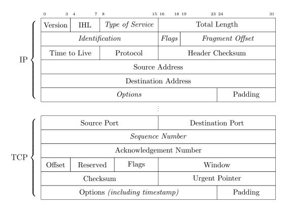
Figure 3.2: Basic TCP/IP header structure
