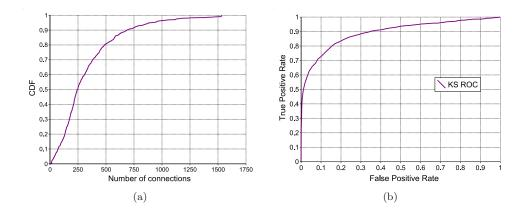
Fig. 4. Client linking in Tor with generic timing. Figure (a) shows the cumulative distribution of timing samples per run. Figure (b) shows the ROC results; the area under curve is 0.89.
