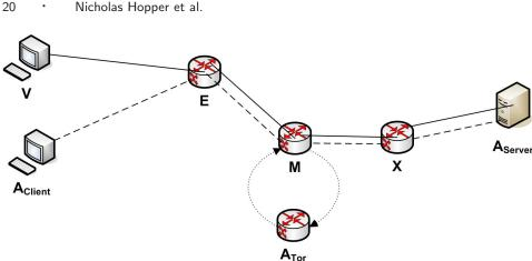
Fig. 11. Tor client location: client V connects to malicious server A via circuit E-M-X; A determines E-M-X and connects to A via E-M-X.
