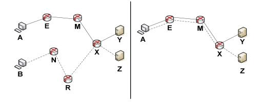
Fig. 3. Circuit linking scenario: client A connects via circuit E-M-X to server Y, and client B connects via N-R-X to server Z. Y and Z collude to determine if A-E-M and B-N-R are distinct (left) or identical (right) paths.
