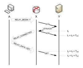
Fig. 1. Measuring Tor circuit time without application-layer ACKs: the estimate for  $T_{AX}$  is  $t_3 - t_1$ . We abuse notation and write  $T_{XY}$  for the one-way delay from X to Y.
