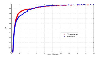
Fig. 2. CDF of circuit times measured by timestamping and redirection.
