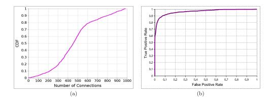
Fig. 5. Client linking in Tor with pipelined timing. Figure (a) shows the cumulative distribution of timing samples per run. Figure (b) shows the ROC results; the area under curve is 0.96.
