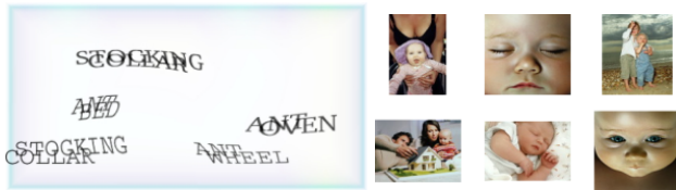
Gimpy algorithm: Try to read the words Pix algorithm: What are these pictures of?
